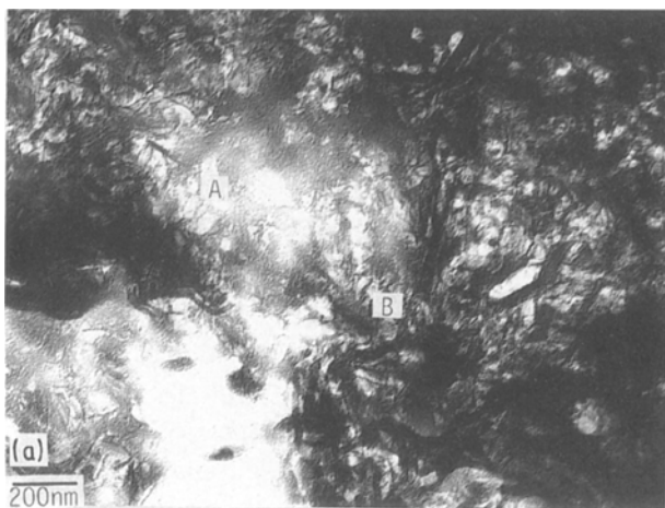
Figure 7 (a) Bright-field micrograph and (b, c) X-ray spectra of a high chromium region of C-S-H in a 1.0 M Cr cement paste. Note, from the X-ray spectra in (b and c), that chromium appears to substitute for silicon.
